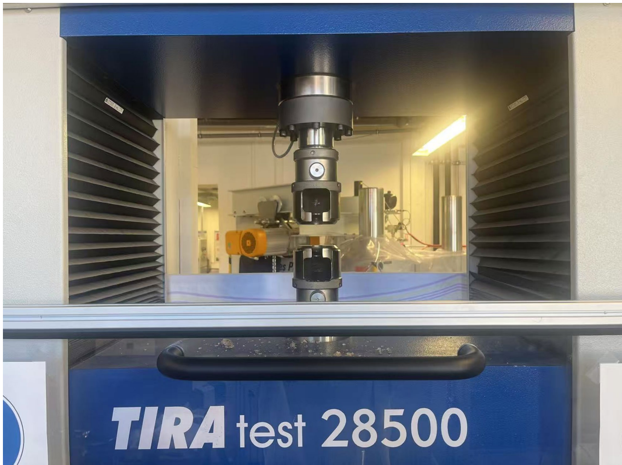
Fig. 1 Compression/tensile testing machine TIRAtest-2800
